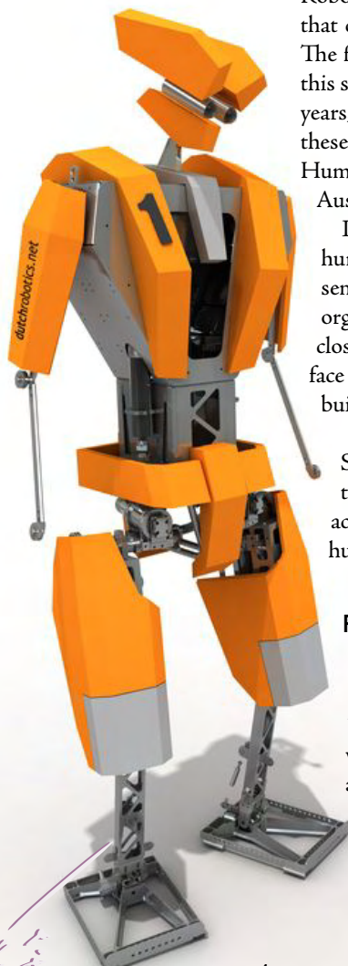
Fig. 1: 'Tulip' humanoid soccer robot
