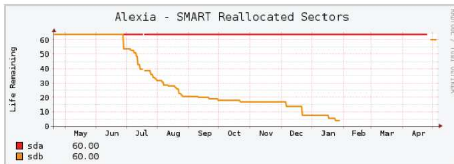
Figure 1: We could have seen that coming. The graphs shows that from June 2012, bad sectors occurred on the drive.
