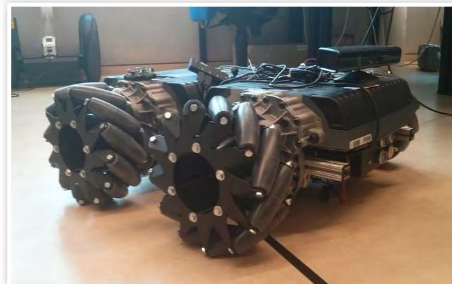
Figure 2: The RMP50-omni platform fitted with the Microsoft Kinect and the appropriate power supply and connections
