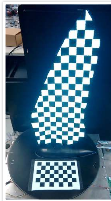
Figure 4: The wing used during the experiments is covered in black spray paint and a retroreflective checkerboard pattern. The corners of this pattern can be tracked with computer vision algorithms. Another checkerboard is placed on the windshield and acts as a static reference frame.
