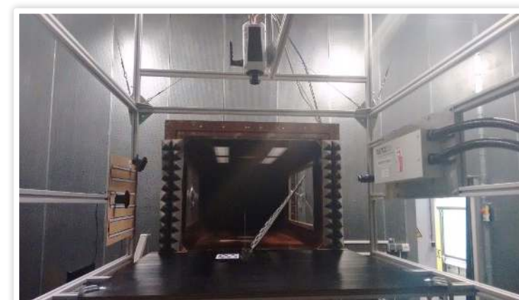
Figure 6: The measurement setup with the wing flapping in front of the wind tunnel. Left: Stroboscope and stereo cameras. Top: PIV camera. Right: PIV laser. The force sensing plate is underneath the black wind shield.
