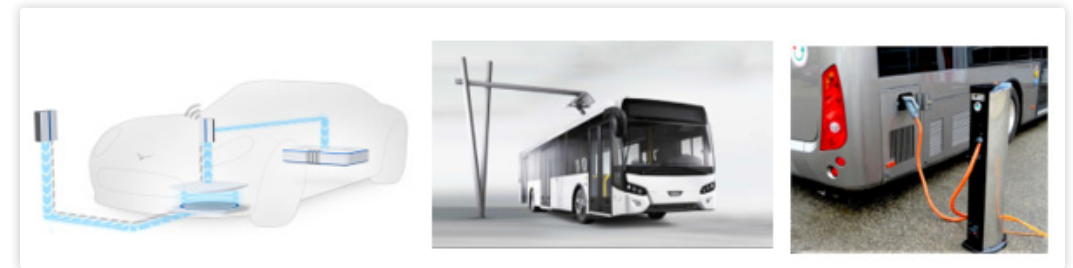
Figure 2: Charging methodology: inductive / pantograph / power plug
