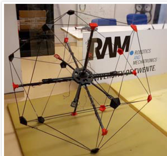
Realisation and implementation of force sensors in a safety cage (without rotors/electronics).
