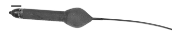
Figure 2: A pop-up satellite archival tag, with antenna on the right which points upwards when the device is floating on the headlike part. Source: [6].
